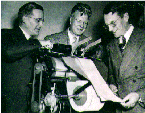
The Xerprinter demonstrated in the late 1940s by John H. Dessauer, Haloid's research head; Chester Carlson; and Haloid President Joseph C. Wilson. This early xerographic device, which printed on rolled paper, commanded public attention, but was never marketed as a product.
