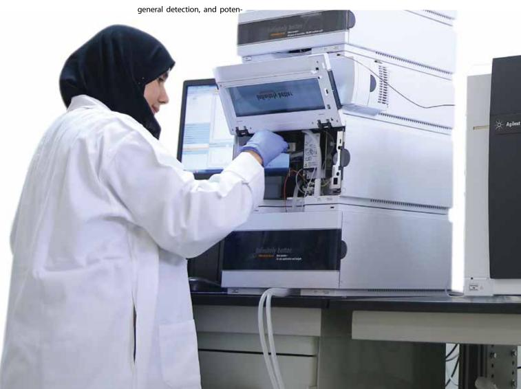
having the flexibility to use up to four different solvents for gradient composition. With power range up to 1200 bar, it can deploy any particle type, any column dimensions, or any mobile or stationary phase.
