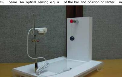
webcam, is used to sense the position and/or the velocity of the ball as it travels along the beam when the beam is tilted. The two end stops of the beam have different colored tags on them, with the ball being in a third color. A control system and software are provided to
