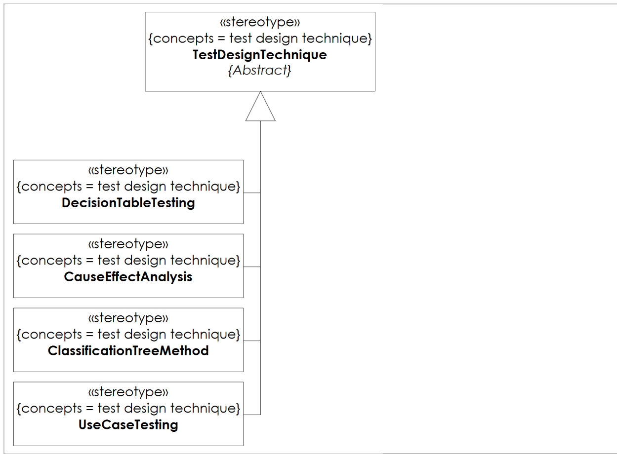
Figure 8.7 - Predefined high-level Test Design Techniques
