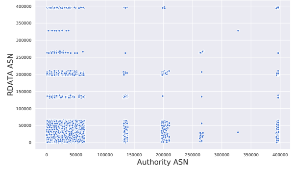
Fig. 19: Scatterplot of the Autonomous System Number (ASN) where the authority’s IP address is being announced from and the ASN where the RDATA for a domain name resides into. The diagonal corresponds to authority-domain pairs that reside in the same Autonomous System.
