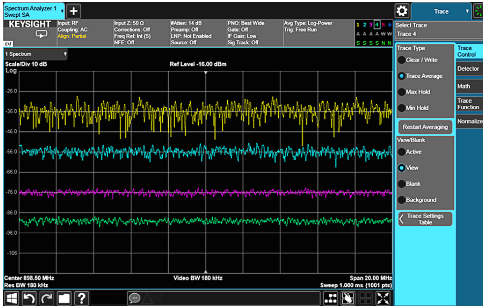
Figure 2-31. Trace averaging for 1, 5, 20 and 100 sweeps, top to bottom (trace position offset for each set of sweeps)
