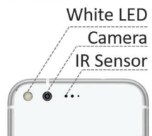
Figure 2: The HemaApp system has gone through a few iterations of improvements. The first version relied on custom hardware. The second version replaces the custom LEDs with a standard white flash LED with a change in the capture algorithm. The newest version attempts to reintroduce IR light by accessing the phone's time of flight IR sensor next to the camera.
