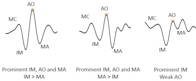
Figure 4. The SCG is produced by the consecutive mechanical movements during a heartbeat (MC, IM, AO, then MA). However, the relative amplitude of each movement changes depending on the person and position of the accelerometer placement.
