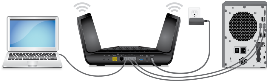
Figure 8. Ethernet port aggregation to a LAN device
