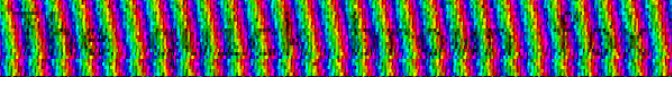
Fig. 1. In this HSV rasterization of the resampled SDR data, prior to approximate frequency correction, the horizontal period length of the rainbow banding is f_s/|f_c - hf_p| samples, and therefore indicates how far away from 0 Hz the nearest pixel-frequency harmonic hf_p is after initial downconversion by the SDR.
