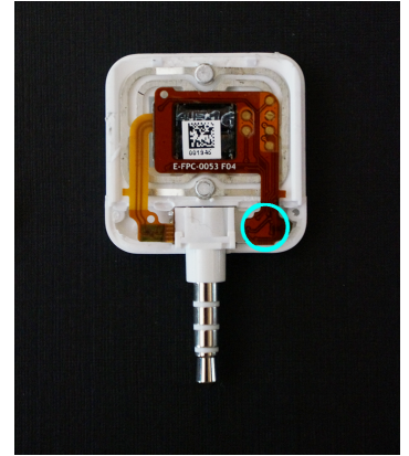
Fig. 3. The location of the model S4 Square Reader encryption chip.
