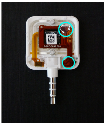
Fig. 4. The model S4 Square Reader with both stages of the hardware encryption bypass implemented.
