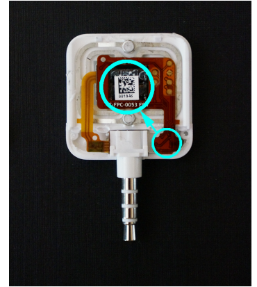
Fig. 6. In order to properly implement point-of-swipe encryption, Square should move the encryption chip to the magnetic head as shown.
