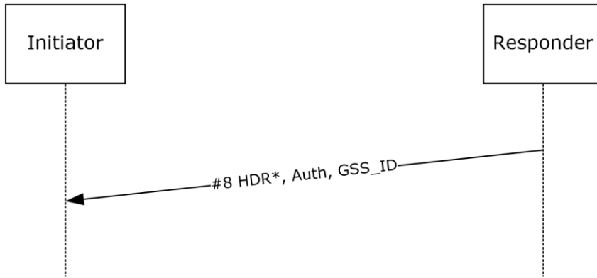
Figure 24: Quick Mode Synchronize Notify packet
