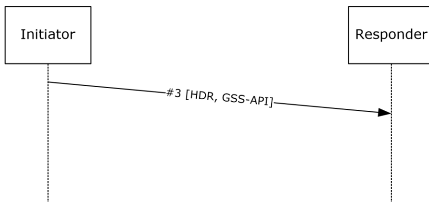
Figure 29: GSS-API initial exchange packet
