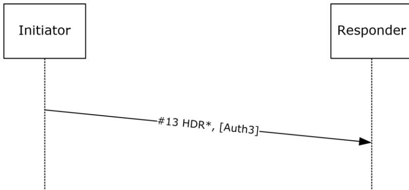
Figure 25: Extended Mode Final Exchange packet
