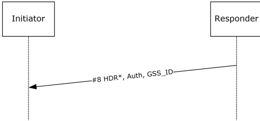
Figure 24: Quick Mode Synchronize Notify packet
