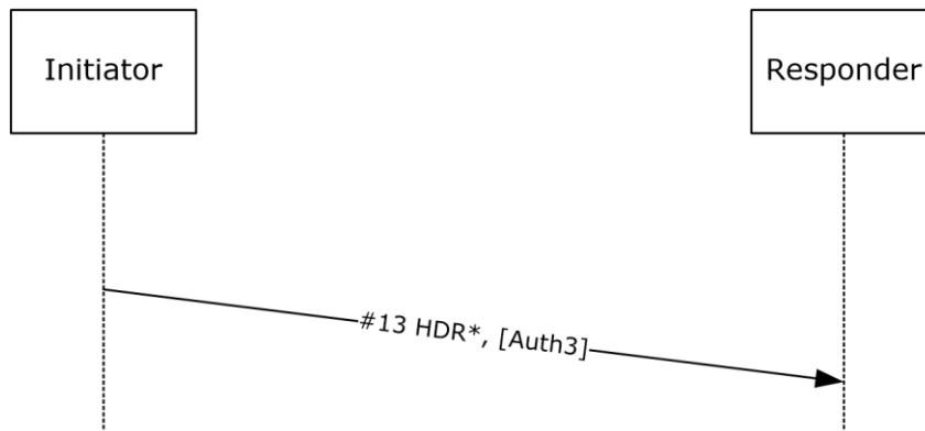
Figure 22: Extended Mode Initiator final exchange packet
