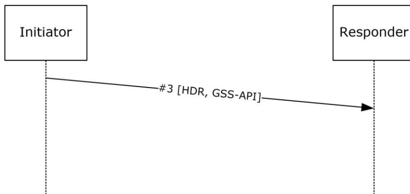
Figure 28: GSS-API initial exchange packet
