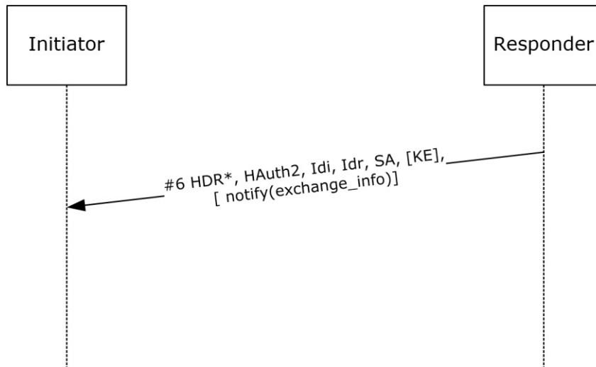
Figure 8: Quick Mode First Exchange Response packet
