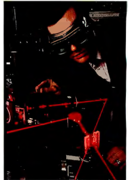
Photo 2: Testing a new polymer that has photorefractive properties. These characteristics may lead to the development of applications such as optical memories or optical data storage many times denser than what is available today. (Photo courtesy of the IBM Research Division, Almaden Research Center, San Jose, CA)
