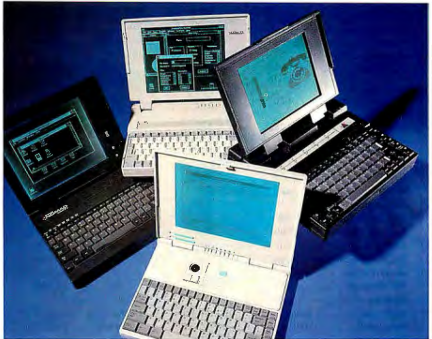
Although slightly bulkier than typical 386SX or 386SL designs, 486 notebooks handle tasks that slower processors can't easily accomplish. Clockwise from left: Gateway 2000's Nomad 420SXL, Toshiba's T4400SX, Ergo's NoteBrick 486, and Compudyne's 4DX/33.
