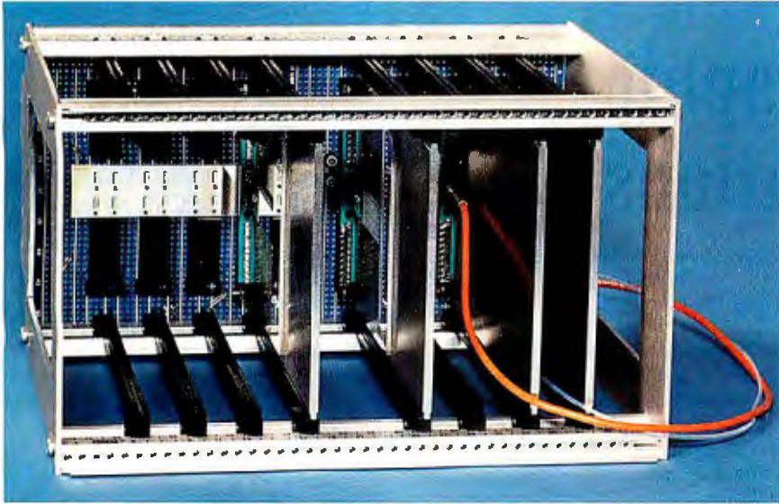
Photo 3: Optical backplane hardware assembled in a VME card cage. Its function is to implement 32 fanouts distributed over four double-sided daughterboards inserted in the four card slots on the left side of the card cage. The prototype device was produced by Charles T. Sullivan, Bruce L. Booth, and Anis Husain. (Photo courtesy of Honeywell Systems and Research Center, Bloomington, MN)
