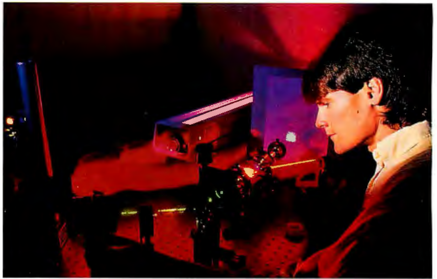
Photo 4: Carl Verber of the Georgia Institute of Technology is building POHMs that can store multiple patterns of data or programs and apply them in parallel to a CMOS array of processors. Here you see Mark Jones, a student assistant, adjusting laser beams in a holographic switching experiment. (Photo courtesy of Georgia Institute of Technology)
