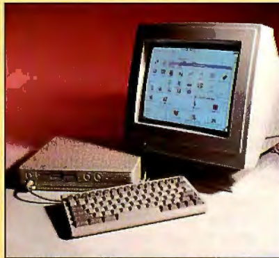
The Addtech SlimPro, a transportable computer similar to the Ergo Brick and the Flytech Carry1, lets you carry your computer from site to site and be able to plug in a full-size keyboard and monitor.
