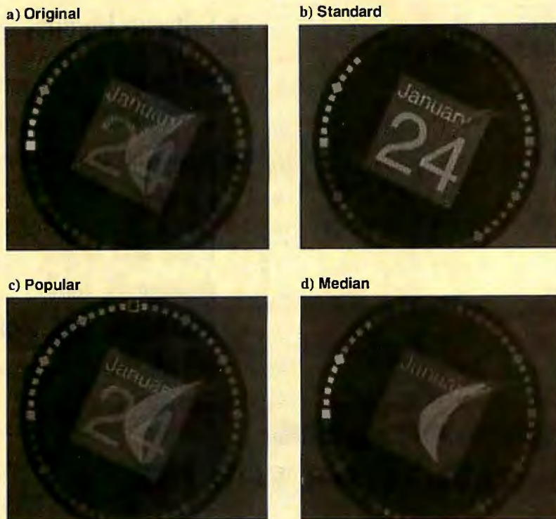
Figure 6: An example of the image results you can expect when using several color-selection mechanisms. (a) is the original image, (b) uses the colors in the standard 4-bit system palette, (c) uses the 16 most popular colors, and (d) uses 16 colors as calculated by the median-cut algorithm.
