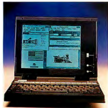
The 50-MHz Model T50 has an optional internal adapter for an external CRT monitor.
