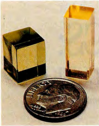
Photo 1: Polymer memory cubes such as these prototypes developed by UCI's Peter Rentzepis are capable of storing information in three dimensions. Data can be written and read in thousandths of a second by two laser beams. (Photo courtesy of University of California-Irvine)
