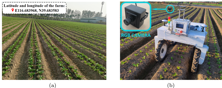
Figure 4: Details of data acquisition. Fig. 4(a) shows the lettuce farm where the data collection took place. Fig. 4(b) shows the setup of the data acquisition process based on VegeBot.
