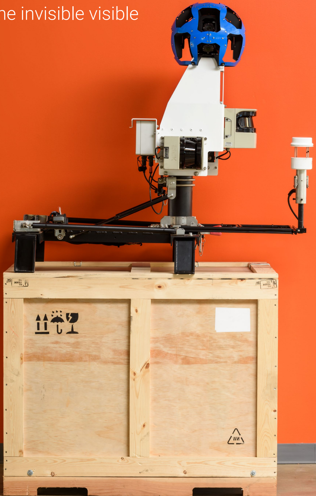
A Google Street View camera fitted with air quality equipment
