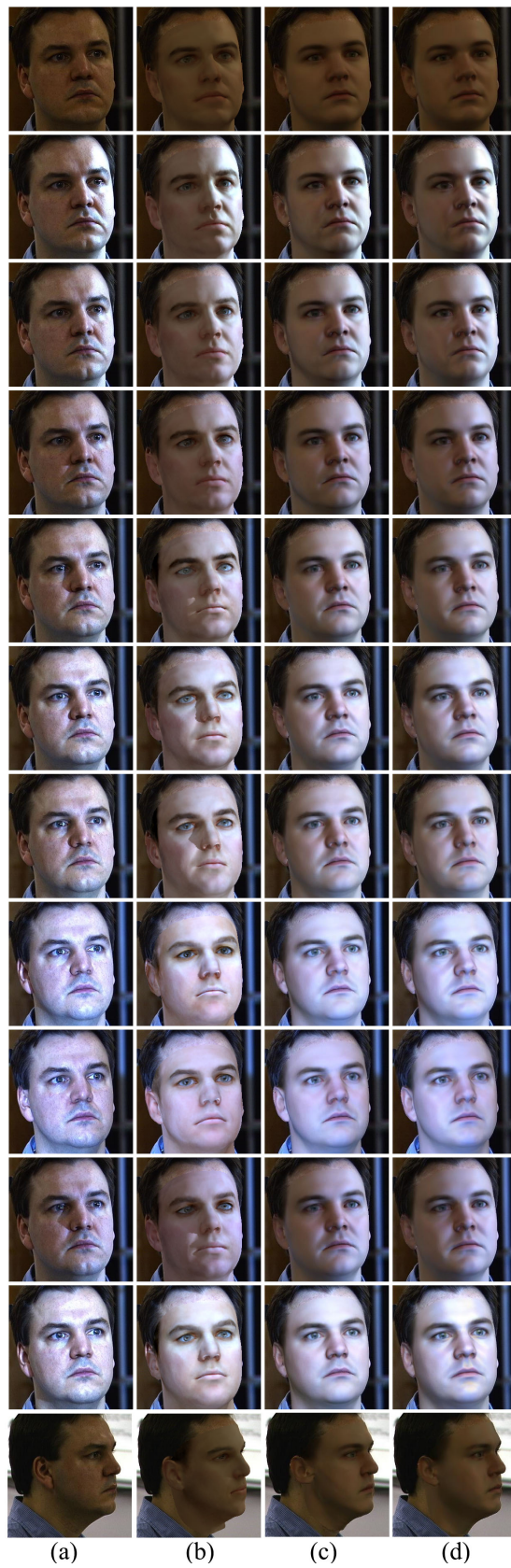
Fig. 3 Comparison of robustness of illumination model to lighting. Columns (from left to right) show: (a) input images; (b) fitting results given by Phong's model [3]; (c) fitting results given by the proposed approach without specular reflectance [2]; (d) fitting results given by the proposed approach.
