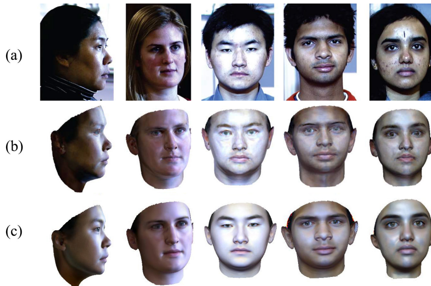
Fig. 1 Comparison of accuracy of recovered shape. Rows from top to bottom, (a): input images; (b): Reconstruction result based on feature points [1]; (c): reconstruction of proposed approach;
