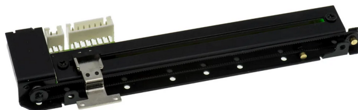
Figure 8: The Bourns PSM01-082A-103B2 motorised slider (image reproduced from promotional material)
