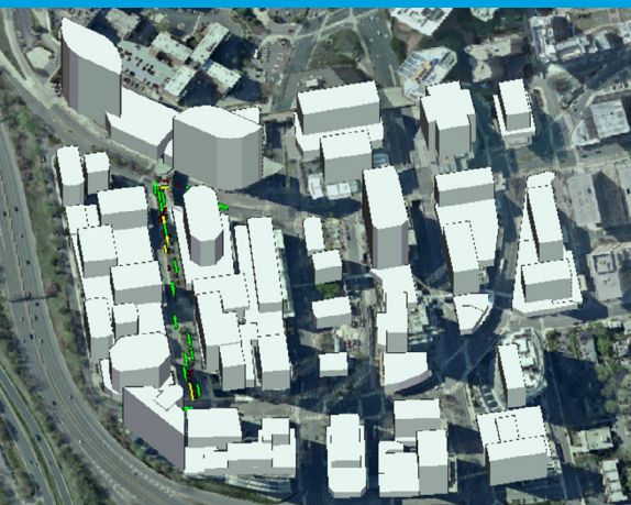
Figure 2 – Example of 3D scenario in which the number of faces was reduced to decrease the ray-tracing execution time. The vehicles are highlighted in vibrant colors in the street under study
