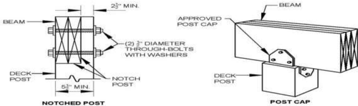
FIGURE R507.7.1 DECK BEAM TO DECK POST
