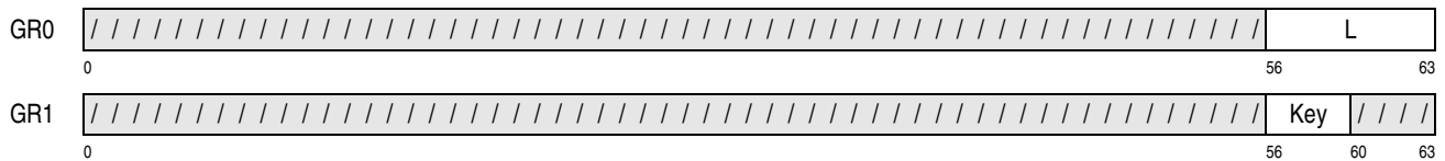
Figure 10-32. Register Contents of MOVE WITH DESTINATION KEY
