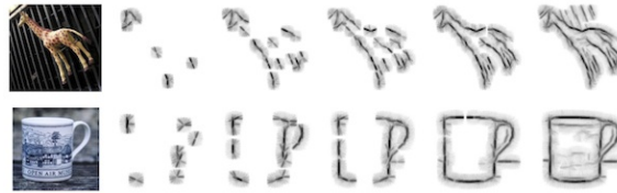
Fig. 3 Shape is robust with respect to missing parts and shape information is predominantly concentrated at points of high curvature. Example sparse shape representation taken from [47].
