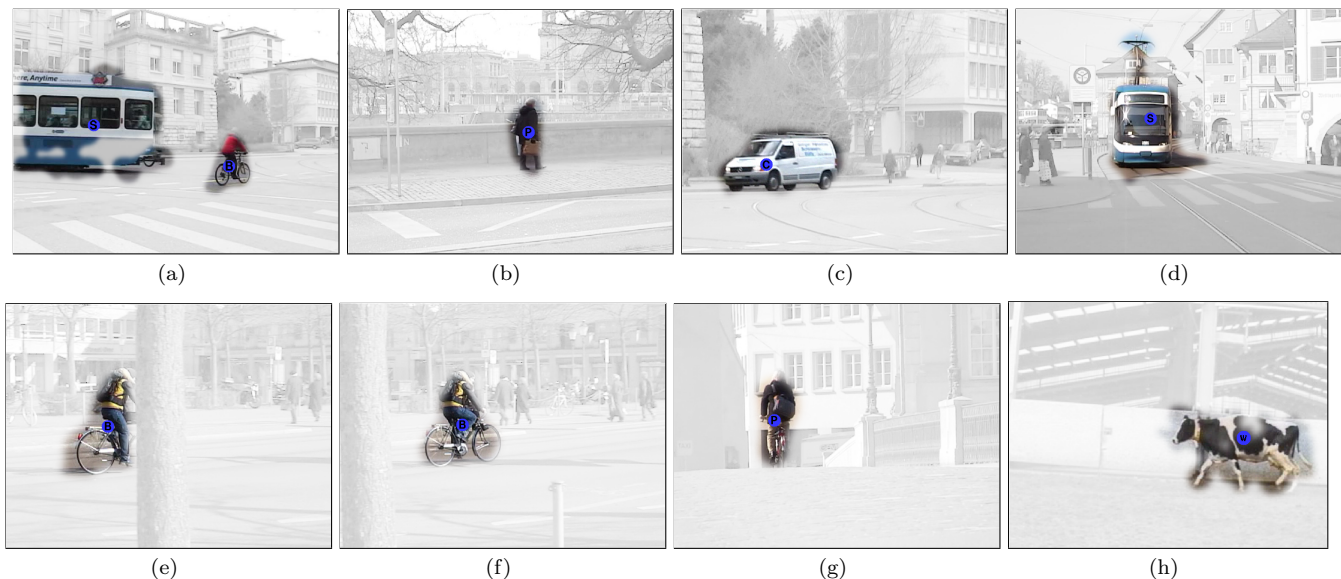
Fig. 6 Segmentations and object categorizations on the dataset of [31]. The category label c^{t,\nu} is placed at the location of the object center \mathbf{x}^{t,\nu} . (a) Simultaneous recognition of multiple objects. (e) and (f) shows object tracking despite occlusion. (g) shows a bicycle that is erroneously classified as pedestrian. (h) is a sample from the database [25] labeled as cow.
