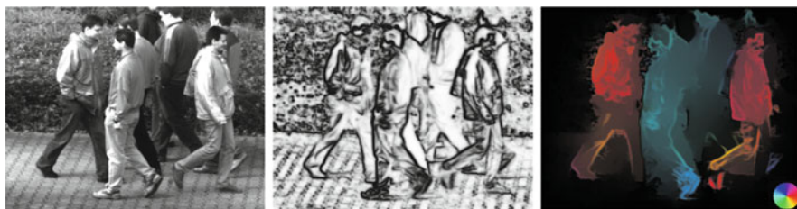
Fig. 5 Pedestrian video: frames from original sequence (left); phase field (middle); optical flow, color coded (right) [114]
