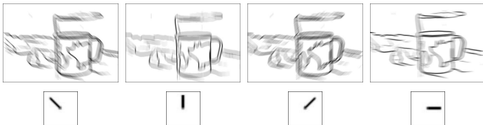
Figure 4: Image edge map convolved with four oriented bar filters. The oriented bar feature is computed by sampling from each channel at interest point locations x_i .
