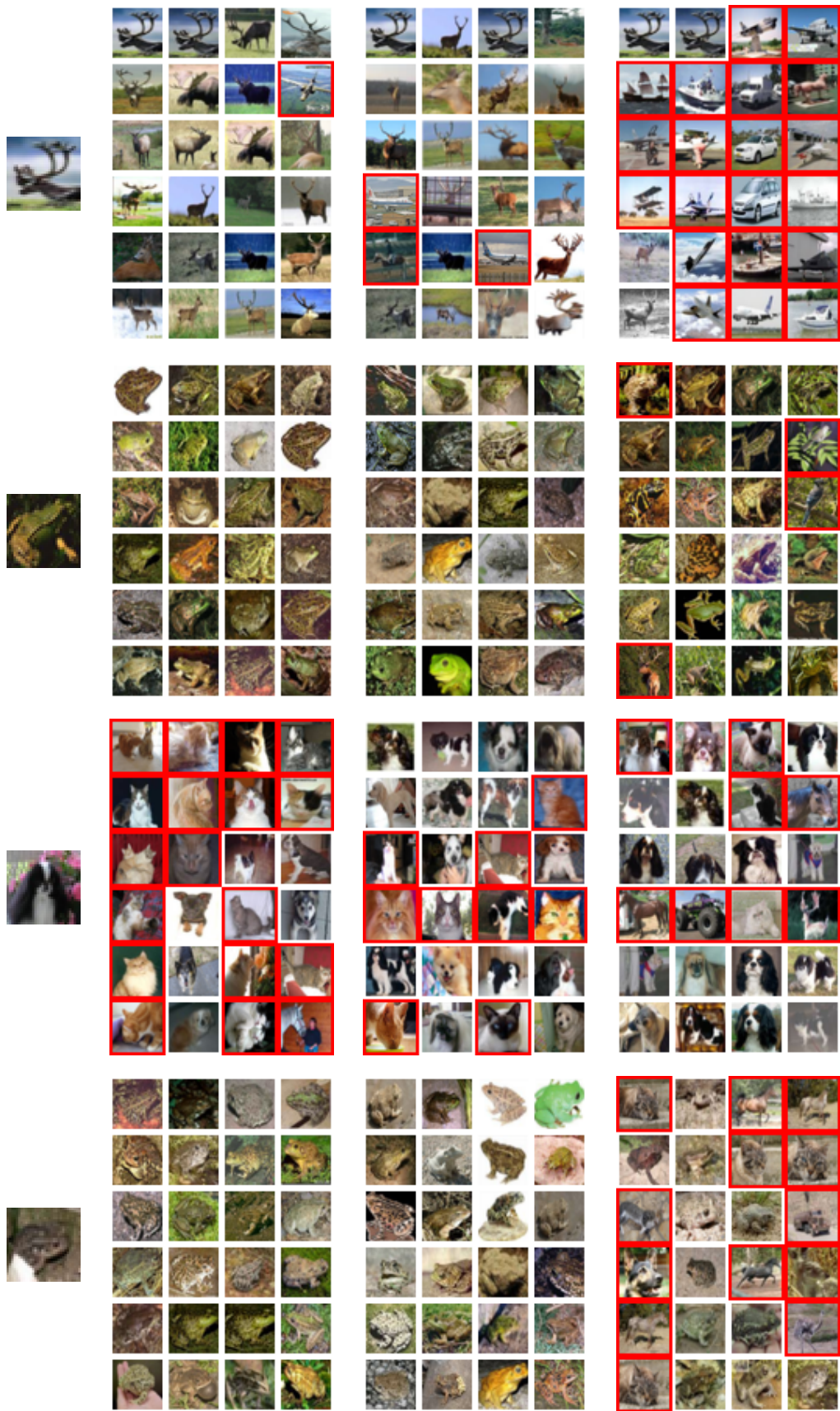
Figure 12: Retrieval results for CIFAR-10 test images 41-44, using Hamming distance on 256-bit and 64-bit codes, and Euclidean distance on bag-of-words features. Red rectangles indicate mistakes.
