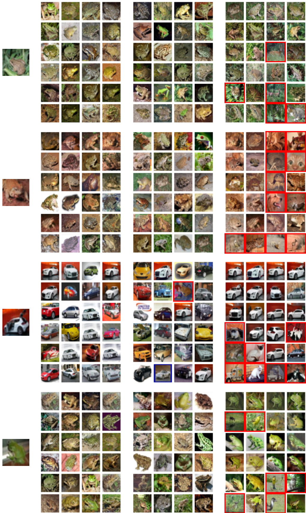
Figure 3: Retrieval results for CIFAR-10 test images 5-8, using Hamming distance on 256-bit and 64-bit codes, and Euclidean distance on bag-of-words features. Red rectangles indicate mistakes.
