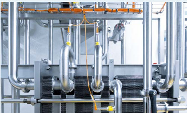
The heart of the plant: plate heat exchanger for precise temperature control of the raw milk
