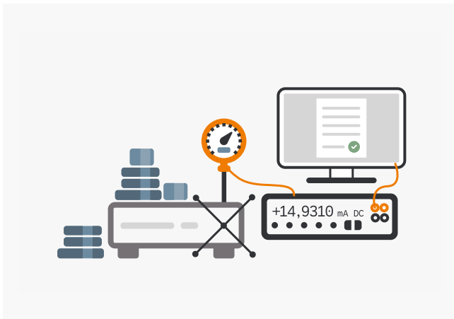
Calibration of pressure gauges by using pressure compensators
