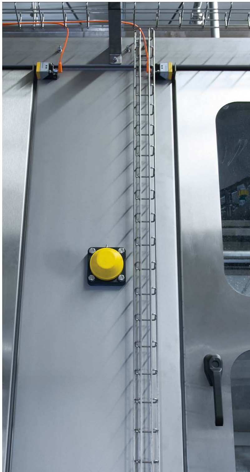
The doors of the system are monitored by fail-safe inductive sensors.
