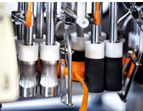
Inductive M8 sensors in a carrot peeling machine
