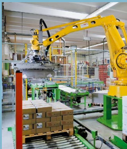
Protective equipment on a packaging robot in a large bakery.
