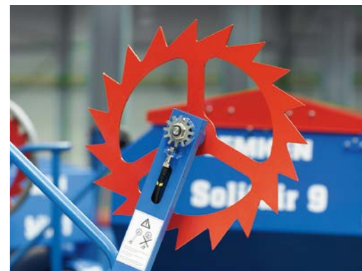
Seed shaft monitoring with an inductive sensor
