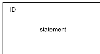
Figure C6.1 - Concrete Syntax for asserted Claim
