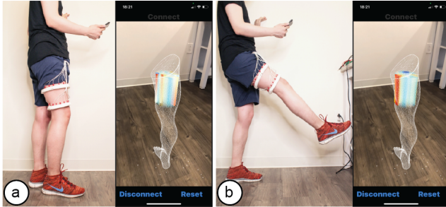
Figure 7: A muscle monitor for physical rehabilitation that can display an AR view of the muscle activity in real-time. Here, the AR visualization shows the muscle activity when the user is (a) standing, and (b) lifting the leg.
