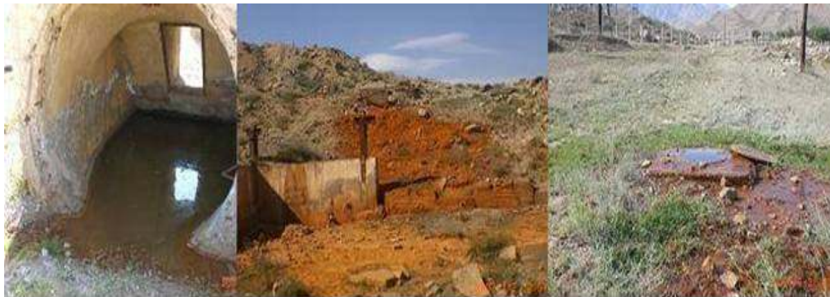
Figure. 29. Mine water draining to the surface via galleries and mine mouth, leaving ferruginous deposits
