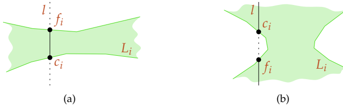
Figure 10.7 (a) The sweepline l intersects a non-vertical bundle in a single interval. (b) The sweepline intersects a vertical bundle in an inverted interval, or lies completely inside the bundle.
