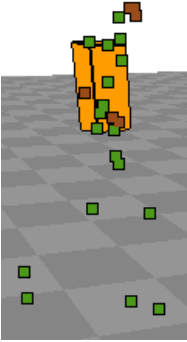
Fig. 4. Finding occluded keypoints using a simple polygon (shown in orange) and the view of the eyes, relative to the orientation of the camera. Occluded keypoints are shown in red, visible ones in green. Note that in our approach keypoints inside the orange polygon are marked as always visible.
