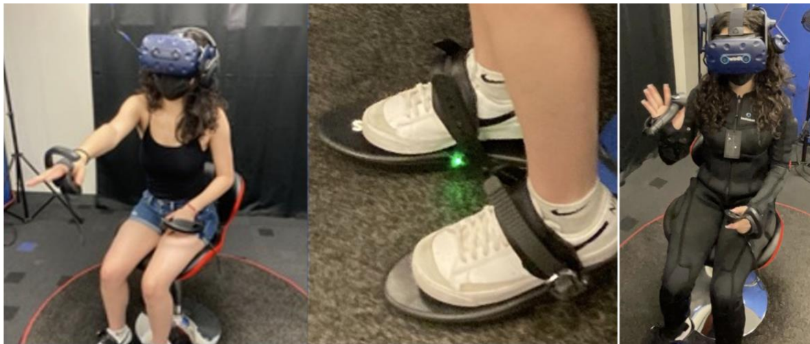
Figure 2: Locomotion via swivel chair ( left ) and shoe interface ( middle ). Right: haptic suit.
