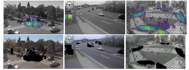
(a) campus (b) highway (c) urban Figure 3: Heatmaps (yellow/blue indicates max/min persistence) and resulting masks for each video in our dataset; persistence range is normalized per video.
