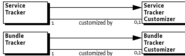
Figure 701.1 Class diagram of org.osgi.util.tracker
