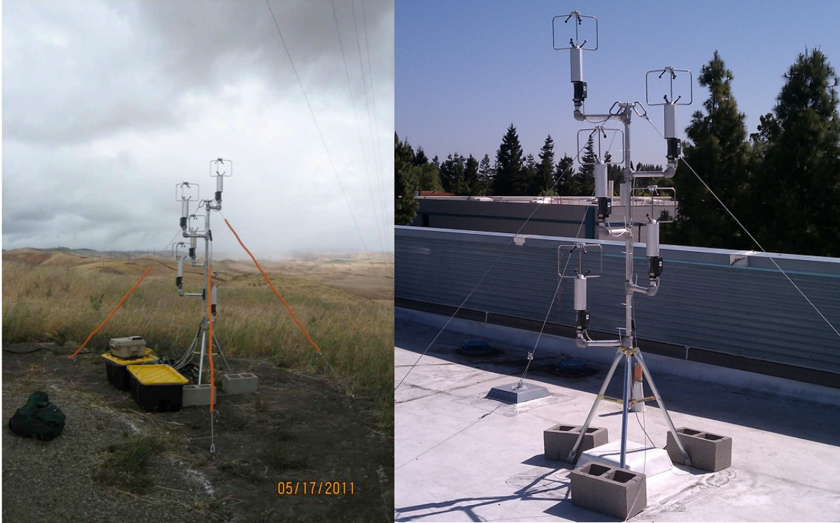
Left: Anemometer array deployed at Tracy site to record atmospheric wind conditions. Right: Similar anemometer array on Google's rooftop lab
