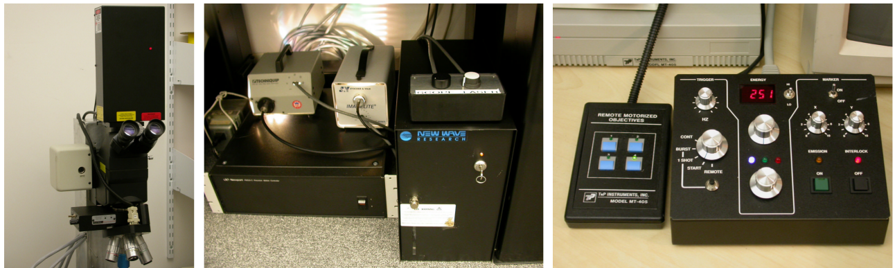
Picture 1. The laser cutting system: a) laser head and microscope; b) control block and illuminators; c) remote controls
