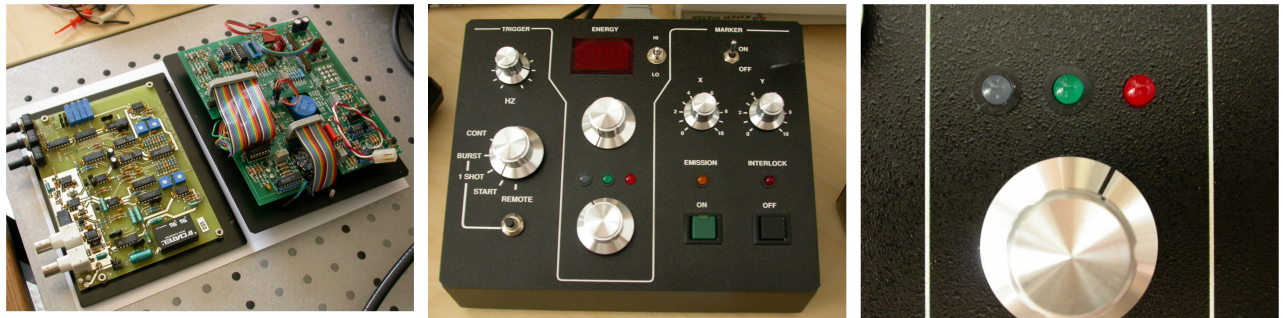
Picture 8. Upgrading the remote control: a) inside view; b) front view; c) close look
