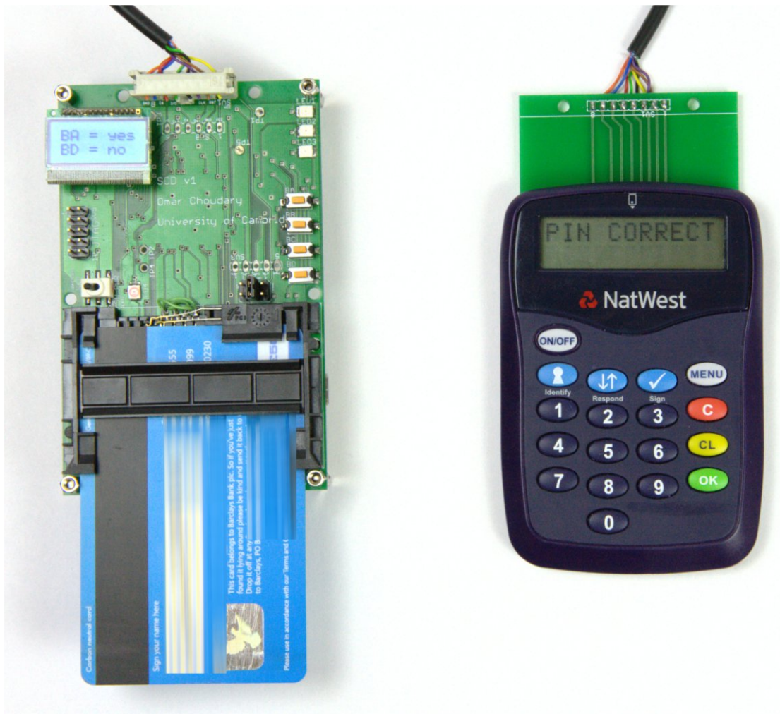
Figure 6.2: Forward Commands application tested on Natwest CAP reader. The SCD has blocked the transaction after the PIN has been entered and is waiting for the user to select if the transaction should continue (yes) or not (no)
