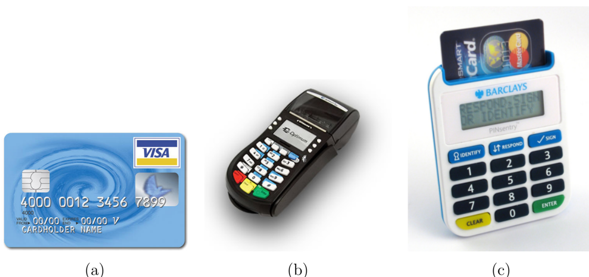
Figure 2.1: Entities involved in the Chip and PIN payment system: smartcard (a), terminal (b) and CAP reader (c)
