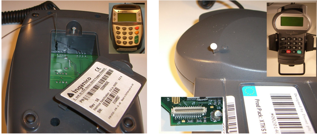
(a) A rigid wire is inserted through a hole in the Ingenico's concealed compartment wall to intercept the smartcard's data. The front of the PED is shown on the top right.
