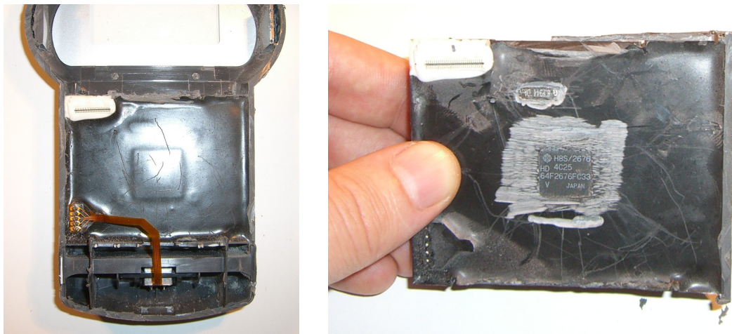
Figure 13: In the potted area of the Dione PED, we can identify the magnetic-strip interface as well as the raised area of the processor and crystal oscillator. The potting was ground down using a rotary tool to reveal the microprocessor – a HD64F2676 H8S/2600 series with embedded 256 kB ROM and 8 kB flash memory – and an 8.2944 MHz crystal oscillator. A sticker covering the processor made the identification process easier. Since the potted area includes the keypad considerable effort would be required to turn it into a fake PED.
