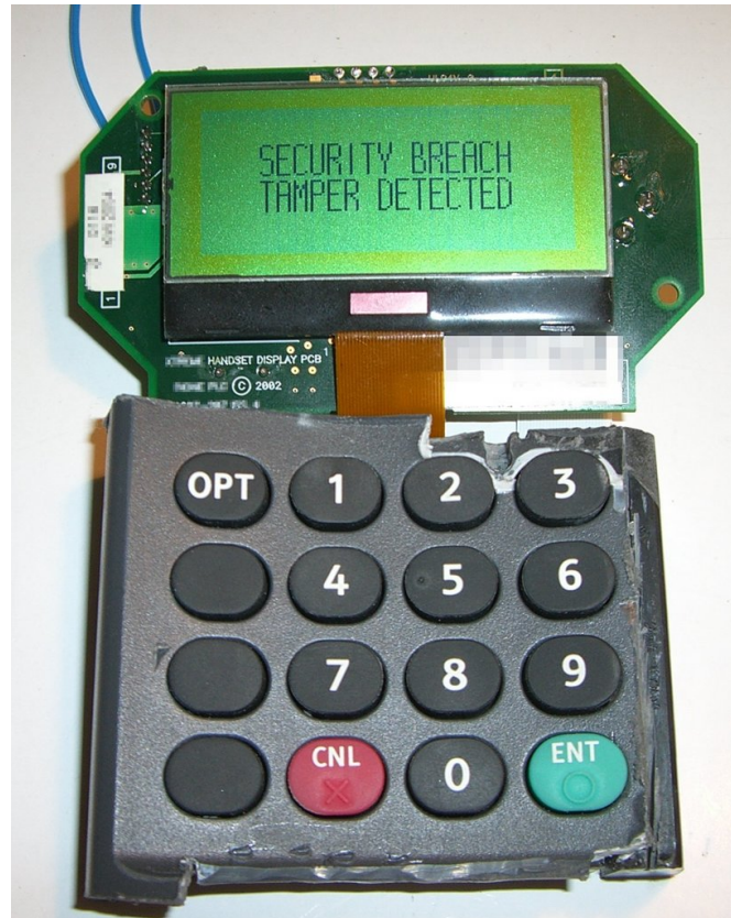
Figure 14: Despite the abuse, the Dione PED still operates and informs the attacker that he needs to move to the next terminal (this alone would reveal how to operate the LCD in case commands are obfuscated). The Ingenico PED simply gives three alarm sounds and ceases to work. It may better to program the keypad so that once online after detecting tampering, it reports the breach. The bank can choose whether to send the police, phone the merchant, or display a innocuous message on the LCD indicating some random fault. In general, it should be hard for the attacker to know whether a tampering attempt has succeeded or failed; such information should cost him as much effort and risk as possible.
