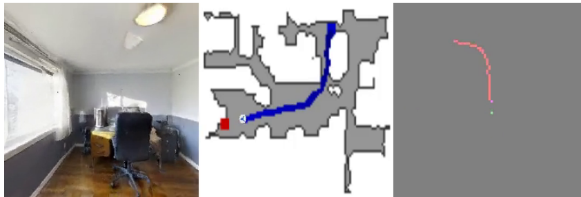
Figure 6: Sample Frame from Local Planning in Habitat. [Left] The agent observes this rgb image. [Middle] Top-down view of the map with boundary information. This map is not provided to the agent and used purely for visualization purposes [Right] From target coordinates provided at every timestep, we can reconstruct a visitation map which we provide the agent.
