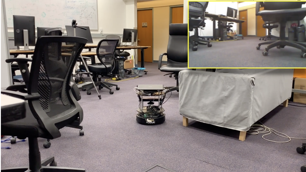
Figure 1: Turtlebot2 navigating to the hallway through a cluttered environment. Agents trained using mid-level vision in simulation successfully navigate in cluttered real-world environments without fine-tuning. The agent’s only input is the RGB frame shown in the top right. See the included video for more.
