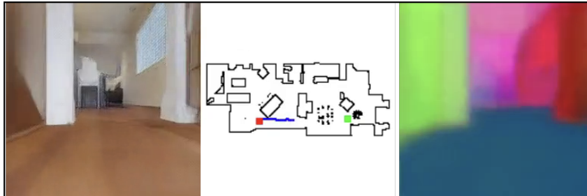
Figure 7: Sample Frame from Local Planning in Gibson. [Left] The agent observes this rgb image. [Middle] Top-down view of the map with boundary information. This map not provided to the agent and used purely for visualization purposes [Right] Visualization of a mid-level feature (surface normals).
