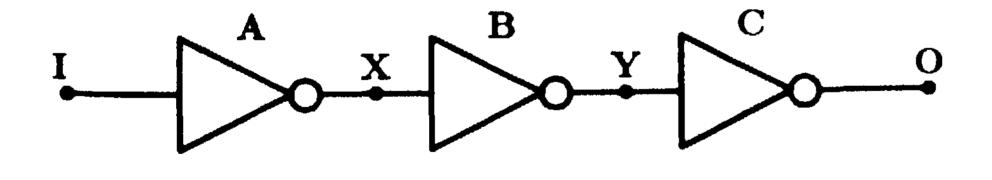
though the output (O) should be one if functioning correctly, it is measured to be zero. Without knowledge of fault modes, all three inverters are equally likely to be faulted. If we knew that inverters (almost) always failed with output stuck-at-1, then we could infer that inverter B was likely to be faulted. Thus knowledge of failure modes can provide significant diagnostic information.
