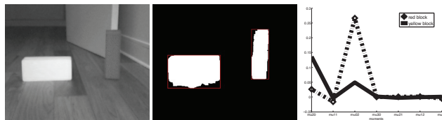
Figure 7: Reuse of visual categories developed for body postures for categorising object positions. This image shows from left to right: the source image, object contours in a binary image, and feature signature of the centralised normalised moments of the two objects in the scene.
