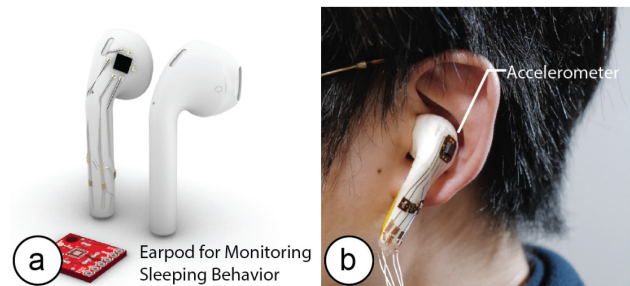
Figure 15. (a) Earpod design in MorphSensor system, (b) non-instructive measurement through an earpod.
