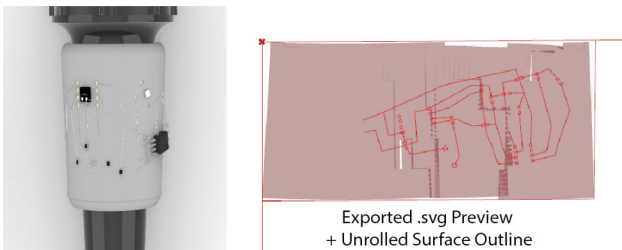
Figure 11. MorphSensor Export for Fabrication.
